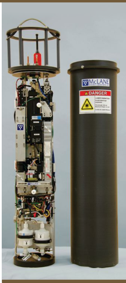
Imaging FlowCytobot (IFCB) is an in-situ automated submersible imaging flow cytometer.
